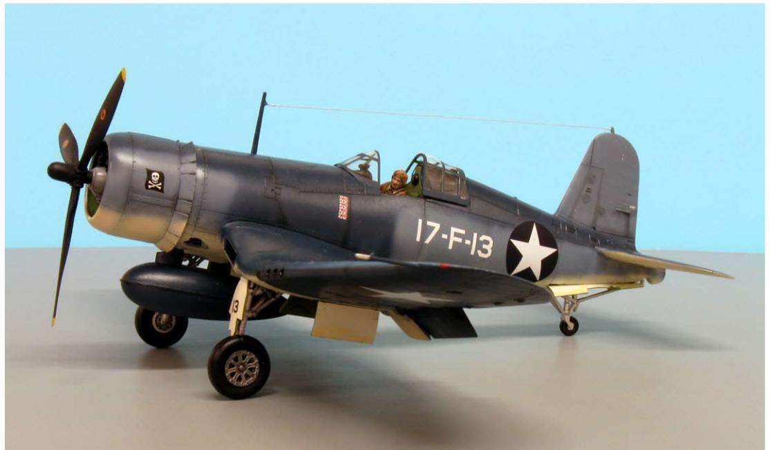
Tim Browning built this nice F4U-1 "birdcage" Corsair OOB from the excellent 1/48 scale Tamiya kit. Tim added copper electrical wire to make the engine's ignition harness. He painted the model with Model Master and Polly Scale acrylics and also used Citadel and Reaper acrylics for hand brushing. The final finish is Future. Decals for VF-17, aboard USS Bunker Hill, came from the kit.
