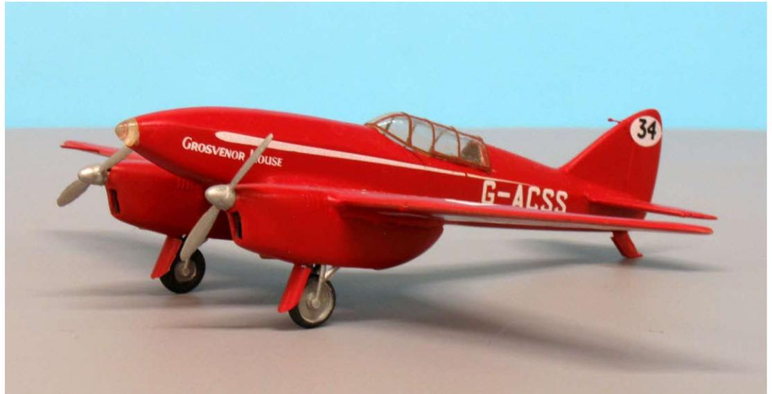
This eyecatcher is Bob Hale's 1/72 scale DeHavilland DH88 Comet, which ranked high on last month's list of the world's most beautiful aircraft. Bob made a new canopy to replace the kit canopy which was a thick, non-fitting affair, added balance weights to the rudder and elevators, removed the solid nose and scratchbuilt the nose landing light, added navigation lights, altered the cooling holes in the engine cowl, and altered the wheel wells. The model was painted with Polly Scale acrylics.
