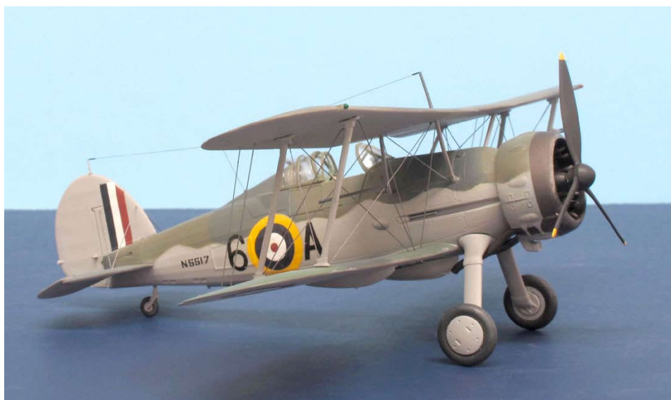
Pip Moss's 1/48 scale Gloster Sea Gladiator. The cockpit was replaced with a resin set from True Details. Paints are White Ensign Marine (Sky Grey and Extra Dark Sea Grey) and Model Master enamels (Dark Sea Grey, Dark Slate Grey and Light Slate Grey). The model was rigged with .008-inch nylon monofilament. Markings (from the kit with Aeromaster roundels) are for a plane flown by Charles Keighley-Peach, Flight Commander of HMS Eagle in the Mediterranean, mid-1940.
