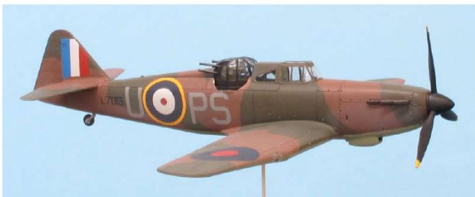
Another factor that contributed to the Defiant being pulled from front line use was the high casualty rate among the gunners, compared to the loss rate of fighter aircrew in other types. To bail out, the gunner had to rotate the turret to point 90 degrees off the aircraft’s centerline, in order to be able to open the hatch on the
